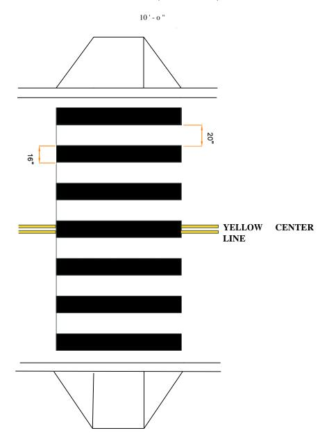
NOTE: SPACING OF LINES SELECTED TO AVOID WHEEL PATH Cross walk shall be the width of existing ADA ramp or sidewalk leading the crosswalk.
